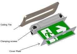
Luminaire Dimensions: 380mm x 220mm
